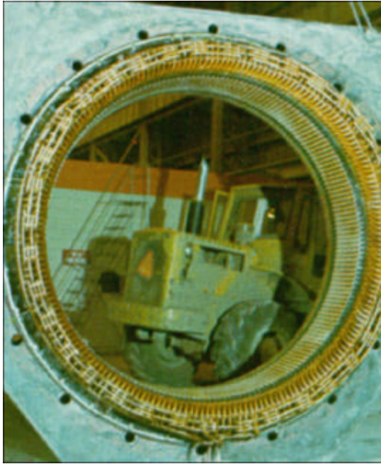
GEGARD tying and bracing procedures reduce winding vibration.
