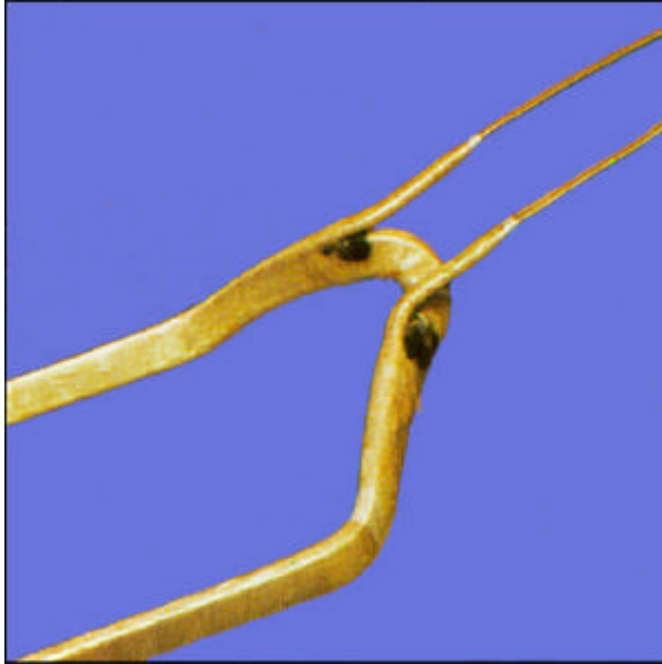
Leads are sealed with a compatible B-staged epoxy pad.
